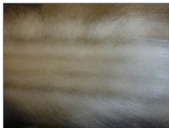
Figure 3. Dynatec die spin pack and a meltblown sample produced using DT2 die design. The top picture shows a Dynatec spin pack made of five little DT2 dies, 1 inch each. The bottom picture shows a web formed with this spin pack exhibiting some non-uniformity (dark areas correspond to low basis weight while light areas represent high basis weight regions). [Color figure can be viewed in the online issue, which is available at wileyonlinelibrary.com .]
